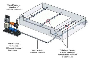
SP sweeper system uses nozzles to prevent solids from settling and "sweeps" them toward the sweeper outlet suction pipe
